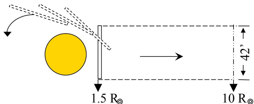
It contains two UV spectrometers (LYA and OVI channels) detecting emission lines in the 950–1350 Å wavelength range. The Table below gives an overview of the UVCS characteristics, for more details see Kohl et al. 1995 and Kohl et al 2006.
