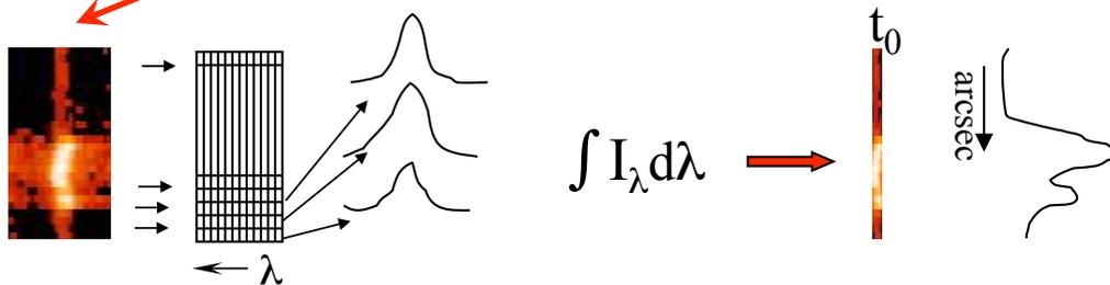
2) Select the spectral line in which CME material is detected and integrate the line profile for each exposure and for each spatial bin to obtain one dimensional images giving the spatial distribution of the line intensity along the entrance slit
