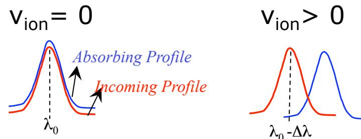
Thus, the line ratio increases and eventually becomes collisional when the outflow speed is such that the absorbing and emitting profiles no longer overlap.
