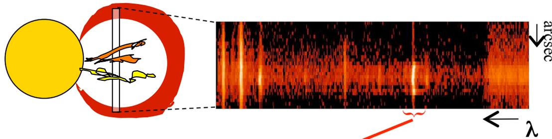
1) As the CME passes through the slit, UVCS collects spectra with a selected spectral range and exposure time
