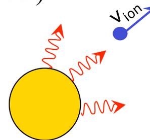
**As the ions move outward in the corona, the radiative component dims because the solar emission and coronal absorption profiles are Doppler shifted apart.**
