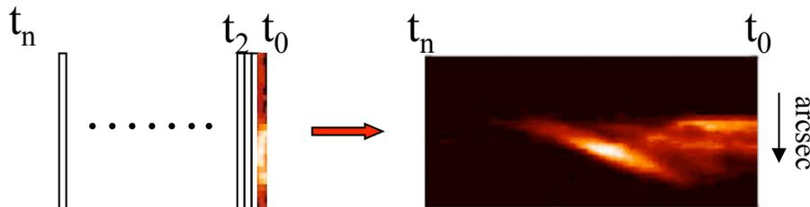
3) By placing the one-dimensional images from consecutive exposures along a time-reversed axis, we obtain an image. The image is then a temporal scan of the event at a fixed position
