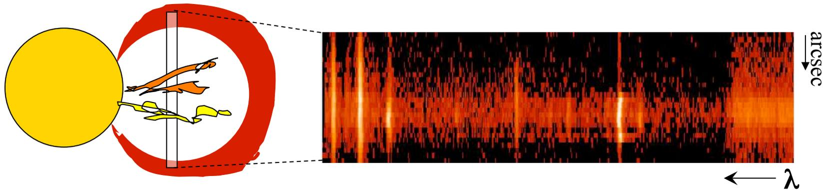
Observation of a CME requires placing the entrance slit at the right time and location in the corona to get spectra of the event as it crosses the FOV of the slit. The spectra are two-dimensional images where the vertical axis is the coordinate along the entrance slit (arcsec or PA) and the horizontal axis is the wavelength dispersion direction.
