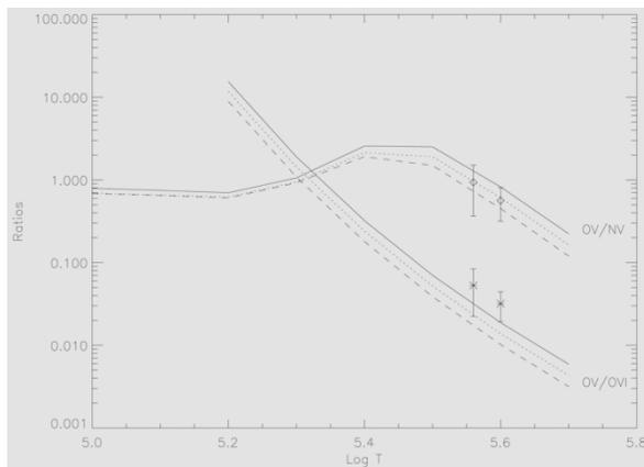
Predicted O V]/O VI and O V]/N V line ratios as a function of the temperature, and density of  $10^6 \text{ cm}^{-3}$  (solid line),  $10^7 \text{ cm}^{-3}$  (dotted line), and  $10^8 \text{ cm}^{-3}$  (dashed line). The diamonds and asterisks are the observed values with their error bars .
